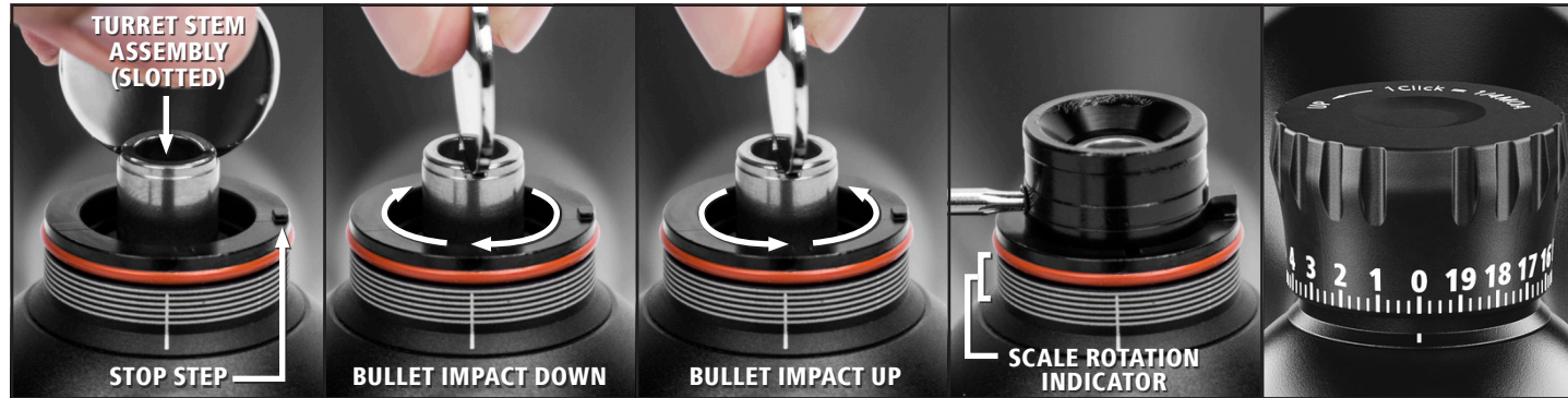
5a. Rotate the slotted portion of the turret stem assembly either downward or upward to your selected zero position.
