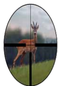
Distance about 100 yards: Image and reticle are located in a single plane (parallax absent).
