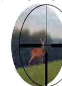
Distance about 300 yards: Image and reticle are behind the reticle (parallax present).
